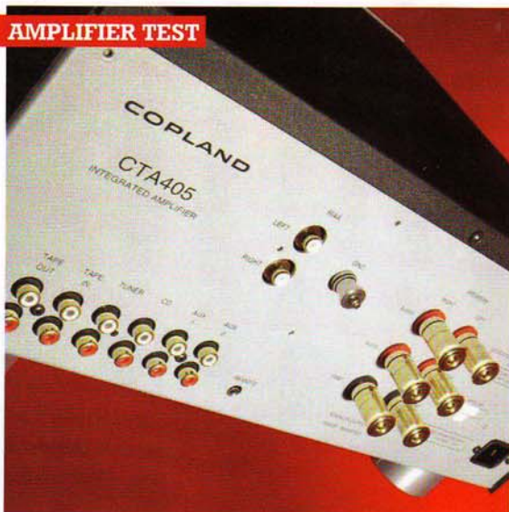
ABOVE: Inputs include four line, a tape loop and a phono stage. Separate 8ohm and 4ohm taps are provided with chunky, gold-plated speaker connections
